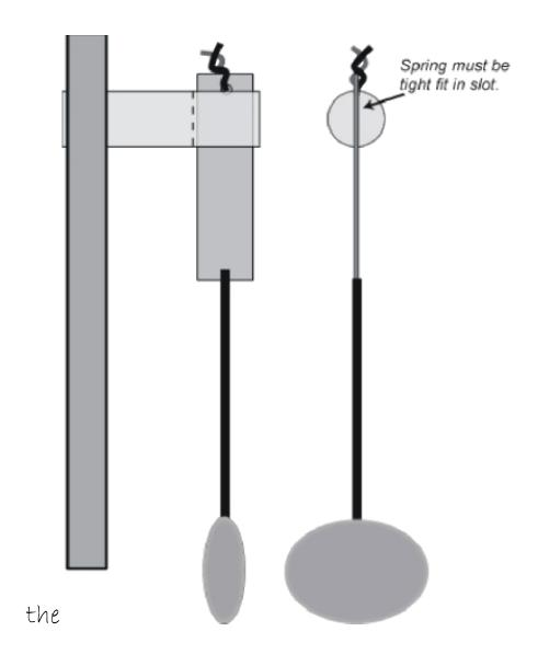
block it could cause the pendulum to wobble and will of course be wasting energy. Some American clocks have a slotted post that the spring slides into and is just held friction tight without a tapered pin or screw. The suspension spring is kept from falling through by means of a small pip at the top of the spring or a small loop of wire which passes through a hole at the top. This spring must also be tight in the slot. Always check to
